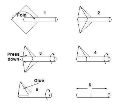
Using a powder flask, put a standard .44 load in the paper, then an equal amount of cream of wheat mixture on top of that. Twist one time, and glue the flap down the side of the cartridge. I usually mark the powder end with a black magic marker.
